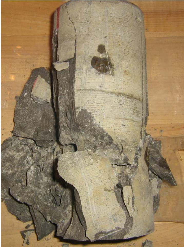
Figure C-5 Specimen DGR-4, 669.90 m
